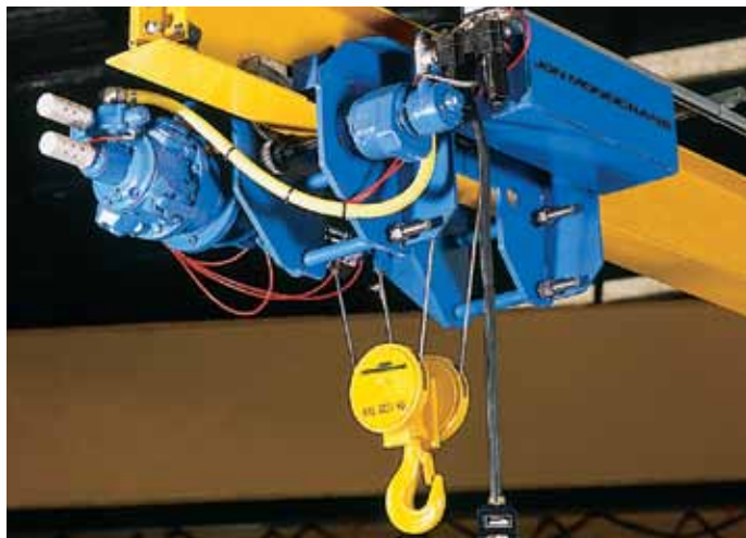
PNEUMATIC HOIST AND LOW HEADROOM TROLLEY
