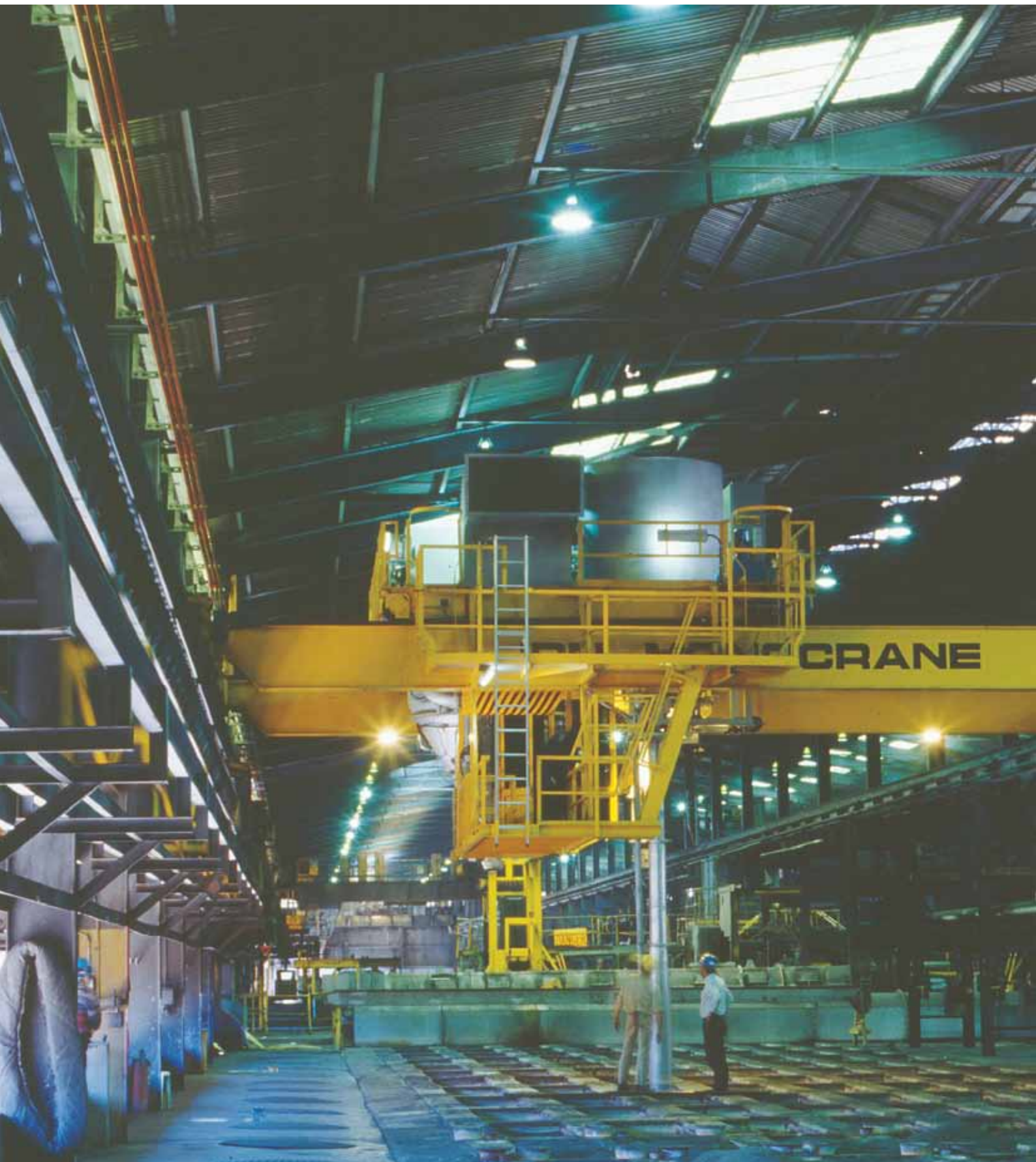
VACUUM CHARGING CRANE IN CARBON BAKE AREA OF ALUMINIUM SMELTER COMPLETE WITH ANODE GRAB.
