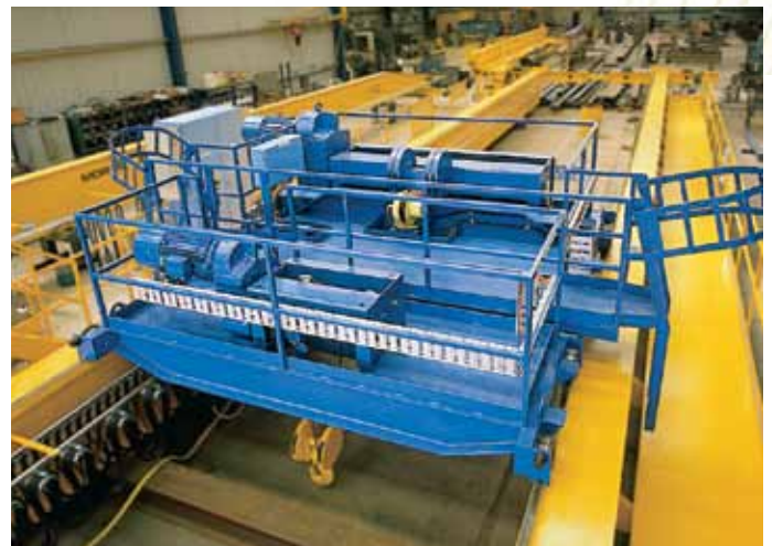
MAIN AND AUXILIARY HOISTS WITH A WALK ON PLATFORM
