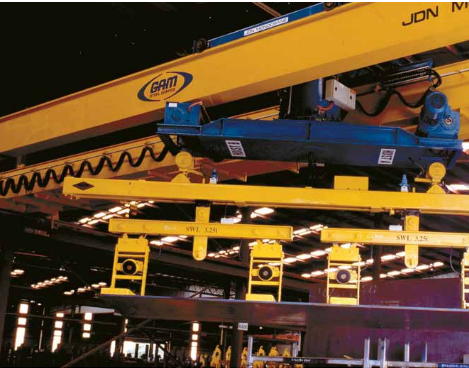
TWIN AH HOISTS WITH MAGNETS AND HYPER SPEED FOR SURE HANDLING
